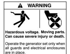
Servicing the generator set when it is operating. Exposed moving parts can cause severe injury or death. Keep hands, feet, hair, clothing, and test leads away from the belts and pulleys when the generator set is running. Replace guards, screens, and covers before operating the generator set
